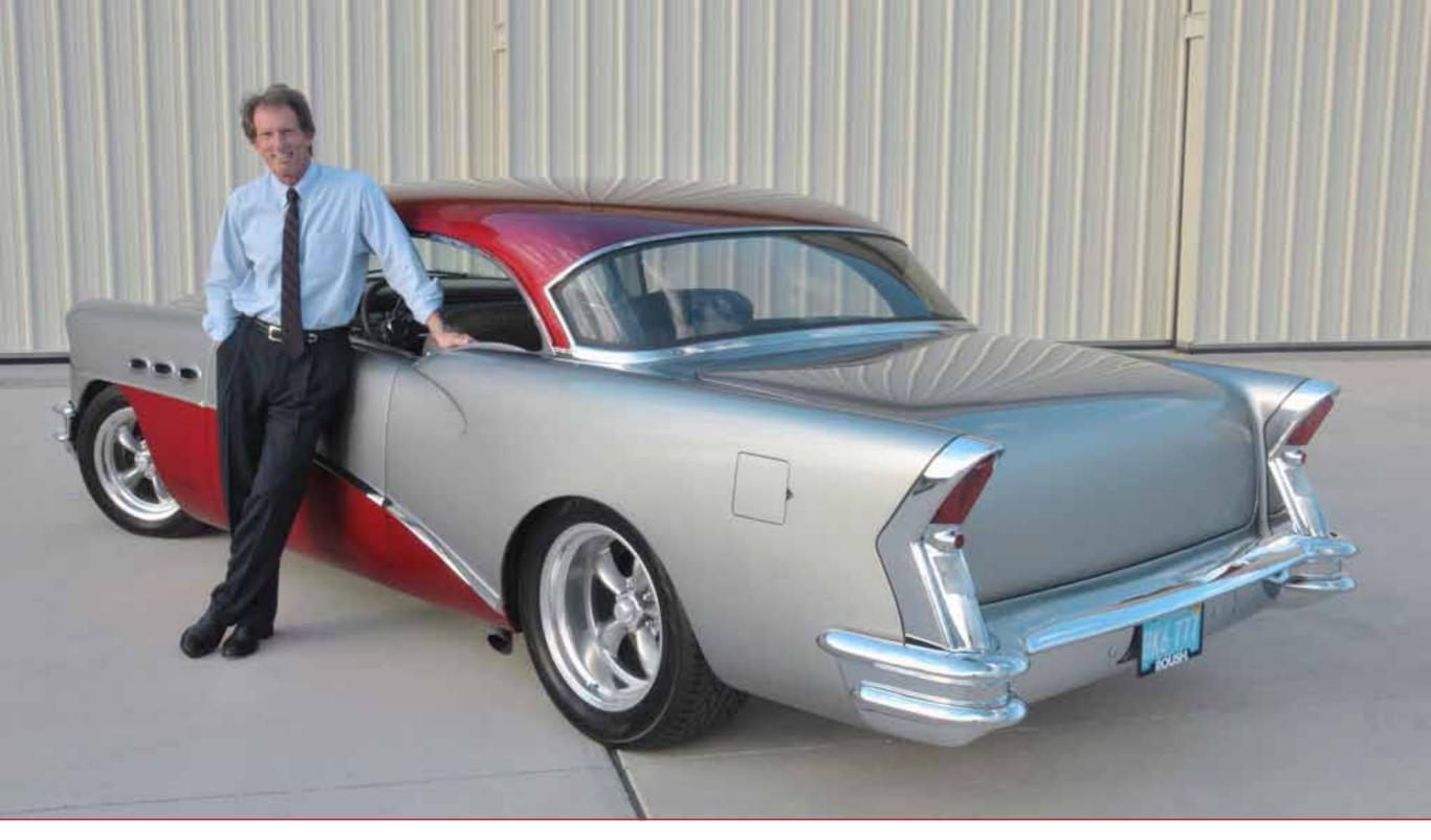
that roughly 30 percent of the chrome on the car has been eliminated. Few, however, will spot the subtleties like the original front bumper shape that has been thinned slightly with approximately one inch of depth removed. The turn signals are now incorporated into the newly minimized bumper guards. The original Buick emblem in the grille was retained but the grillwork behind it was sprayed body color. Factory chrome headlight rims were eliminated and halogen bulbs turn night into day.
